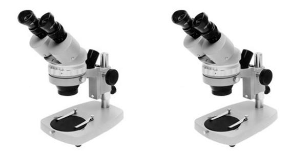
Evidence can be observed simultaneously via the precision engineered comparison bridge that supports two sets of matched objective steps on a 5-step magnification changer.
